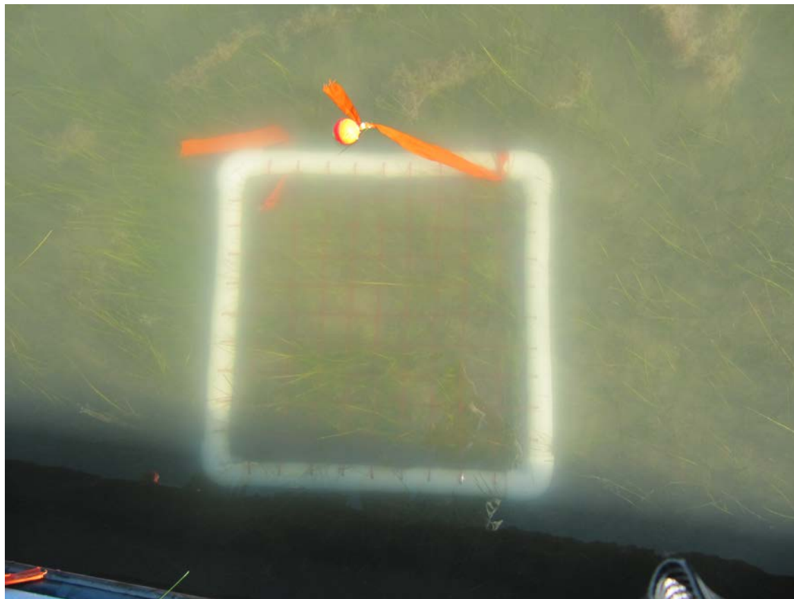
Appendix B - Figure 2. Quadrat for determination of percent coverage by seagrass species. Quadrat is 0.50 m by 0.50 m (0.25 m 2 ) and constructed of white PVC.
