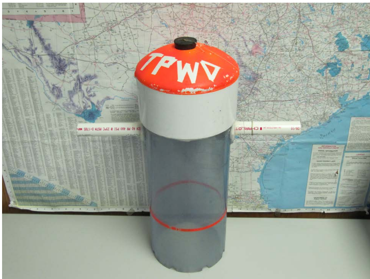
Figure 10. B2.6. Seagrass corer (15 cm inner diameter) used for sampling Thalassia .
